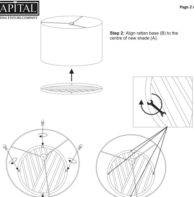
Step 3: Now, Tighten screws (C) on all 4 sides in clockwise direction by using wrench (D).
