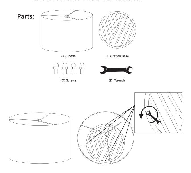
Step 1: Unscrew all 4 Screws (C) from old shade (A) in anti-clockwise direction using wrench (D).
